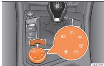
Fig. 173 Console centrale : Commande rotative (Driving Experience button).
